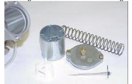
Figure # 6 – The top end parts are accessed by removing the two screws on the Carb top plate.
