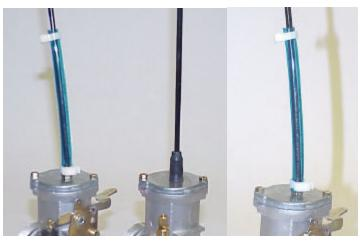
Figure #9 – Special attention needs to be given to the Carb top entry. The use of a short length of ¼" i.d. fuel line makes and excellent strain reliever.
