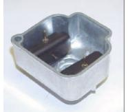
Figure #2 – The float level should be ½" or about 13mm from the top of the bowl with the floats removed.
