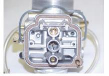
Figure #3 – With the float arm removed you can now inspect the passages including the inlet seat and jet passages.
