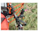
The throttle cable must be outside the white steel cable during flight! It is more comfortable to unbutton the brake line handle from the
