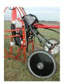
Being alone it is easier to put the engine onto the engine mount by raising the front wheel of the Flyke, until the engine mount is low enough to take the motor hooks. So the engine can be easily attached.
