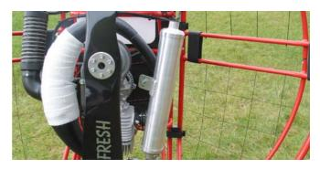
To keep the exhaust flexibly mobile we chose different types of fixtures. One is a rubber connection on the gear-plate and two a stress-bearing spring-gasket at the entry and the exit.
