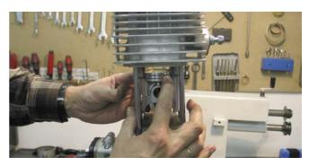
To tighten the headscrews with 14 Nm.
