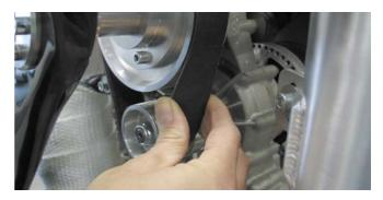
From time to time use the beltdressing. Only one time spaying on the lower pulley is necessary.
