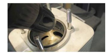
Bore until the drill looks into the outlet-channel.
