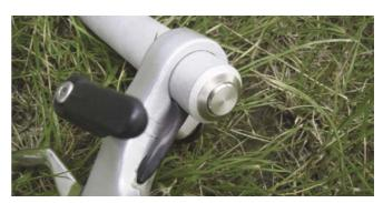
The thottle has also a travelling locking. After reaching the desired hight of flight, the throttle can be fixed via the clasp-lever. Since long holt of the throttle is hard in hand, the throttle can be placed in position onto the legs. The hand are now free for other things.
