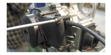
Remove the complete ignitionbox including the lid of the starter. Now the rotor with the starter-pot is visible which is held into place by it's central screw.
