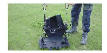
The harness is secured via 3 springlocks; tow legs spring and one breast spring lock. It has two adjustments possibilities. One there are the buckles which are fastenen onto the front of the seat.. At the start these should be pulled on lightly, as to make the climbing into the harness easier at the lift-off. Before landing it is advisable to lower the seat fully, to enable a maximal favourable touch-down position. The leg loop does not need to be pulled too tightly.
