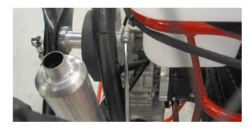
Inside the propellerhub is an allan key-screw. Turn this with the 12 mm allan key until the tension is reached.
