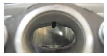
To mount the cylinder you have to press the two pistonrings into the notch.
