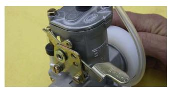
The big screw regulate the idlerunning. Turning right-high rpm. Turning left lower rpm. The idlespeed should round about 24 0 1/min. The smaller screw is responsible for fuelmixture in idle. Turning right-rich. Turning left-lean
