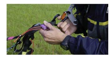
After all has been done, the throttle and the break-loop had to be taken into the hand. The engine will now be started and the starting run can begin.
