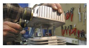
After removing the cylinder you can see the piston. Before you pull out the gudgeon pin remove the safety rings on both sides. Than press out the gudgeon pin.
