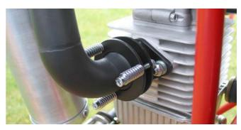
After 10 hrs the sealing-rings and their fasten screws needs to be checked. The screw you have to changes each  $25\ hrs.$
