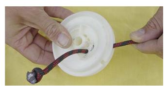
To give the starter-rope advanced tension one, place the rolled up into the slot and rotate three times.
