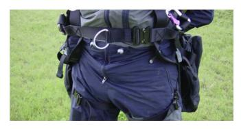
All other adjustment options are regulated while flying. Are the straps pulled rigth and left, then one sits up straight, are they loose a slight back prone position can be adopted.
