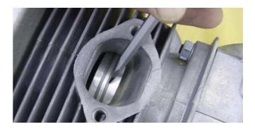
How to replace the piston? At first remove the four nuts from the feed of the cylinder.
