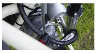
How I change the needle? Open the lid with the two screws and pull out all parts which are hanging on the cable.
