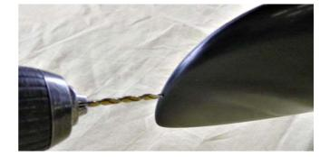
**Attention:** An imballanced propeller created unnessecary vibration in the engine and can destroy many of it's components.
