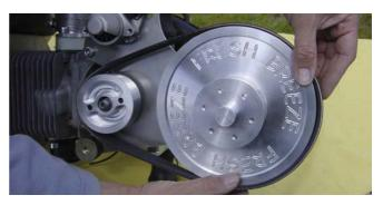
7. Place the new belt onto the pulley.The re-fitting happens in the revrese order.
