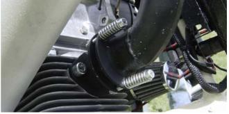
The complete exhaust is suspended flexibly as to prevent vibrational eruptions.
